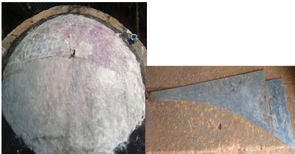
Fig 2: A mould with FRP materials to form the concentrator and a scraper.
